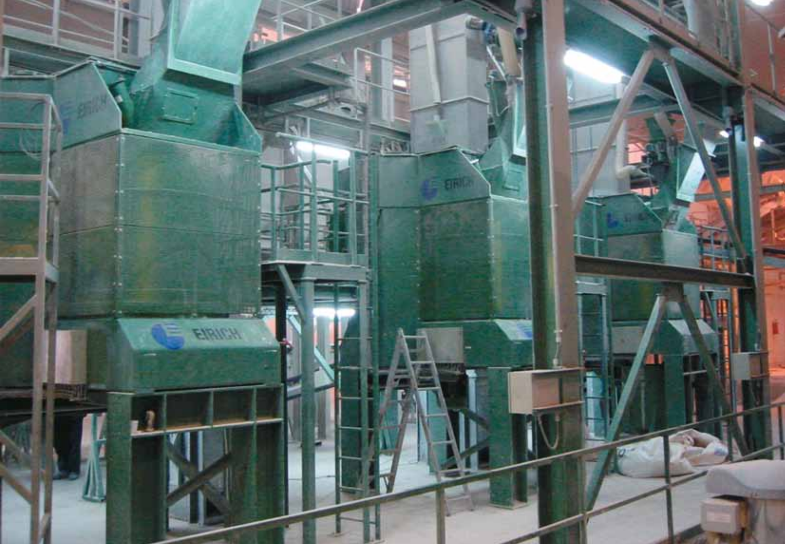
MM5 for dry grinding of hard materials for wall and floor tiles
