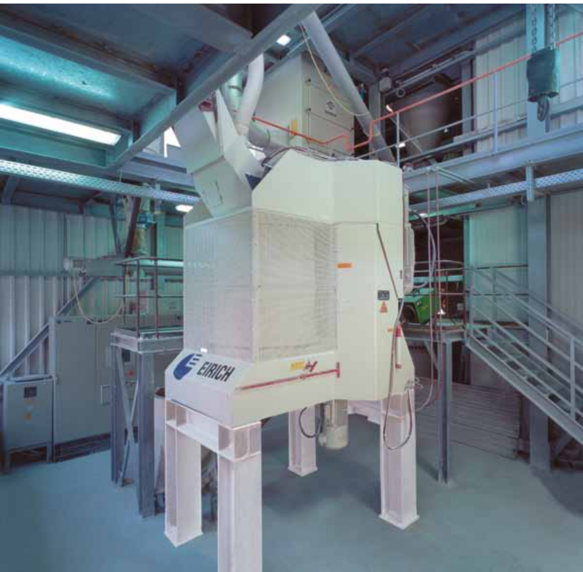
MM5 for dry grinding of hard materials for wall and floor tiles
