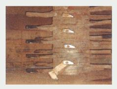
Interior view of an Eirich sinter mixer Rotor after 3 months of operation
