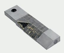
Tungsten carbide faced with a tungsten carbide end piece Production of hardfacing: hard-soldered in our own workshops **Properties**:
