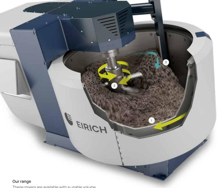
These mixers are available with a usable volume ranging from 1 liter in a laboratory mixer to 12,000 liters in a production machine.
